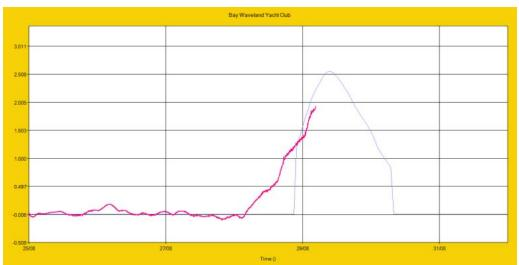
Figure 16 - Blue curve is the calculation and the purple curve is the sea level (measured level – predicted tide) in Bay Waveland Yacht Club
